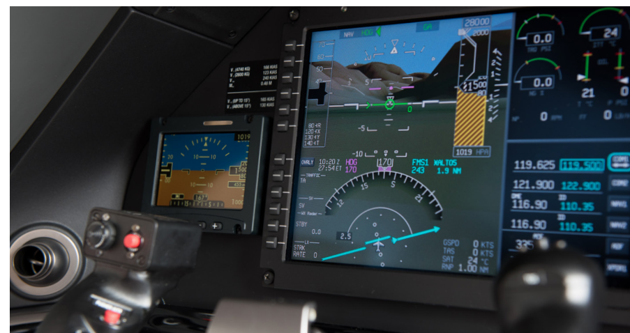
The SmartView™ Synthetic Vision System improves terrain/obstacle awareness by enabling early recognition of conflicting terrain and obstacle, particularly during instrument approaches.
