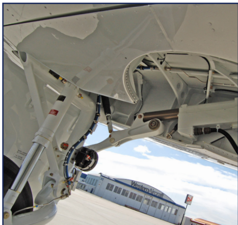
New Electro-Mechanical Landing Gear
