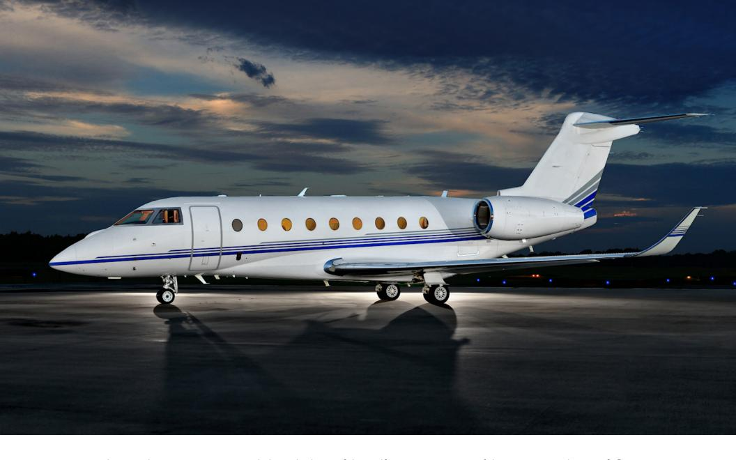
The G280's wing was engineered along the lines of the Gulfstream G550, one of the most versatile aircraft flying today. Because of the exceptional design, the G280 wing needs no leading-edge devices to aid low-speed maneuverability. Instead, subtle contours along a highly swept, smooth wing reduce drag and enhance lift.
