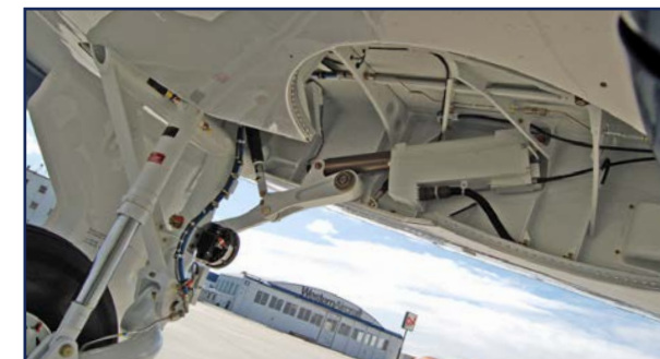
New Electro-Mechanical Landing Gear
