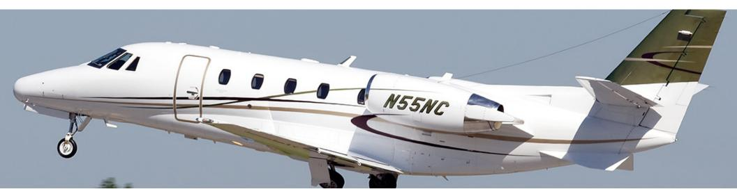
The XLS outperforms competing private jets due largely to its two Pratt & Whitney PW545B engines, designed with a high-pressure core to increase thrust to 3,975 pounds apiece - 4.5 percent more thrust than the engines used in the Citation Excel. These engines can reach 433 kts and have a specific fuel consumption of just 0.709 pounds per hour.
