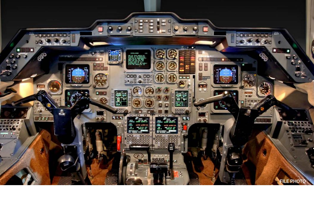
The Honeywell SPZ-8000 Platform features the upgraded RMU-855, Honeywell TCAS-2000, and Honeywell Mark VII EGPWS, covered by Honeywell's Avionics Protection Plan (HAPP). The Hawker is ADS-B v2 compliant.
