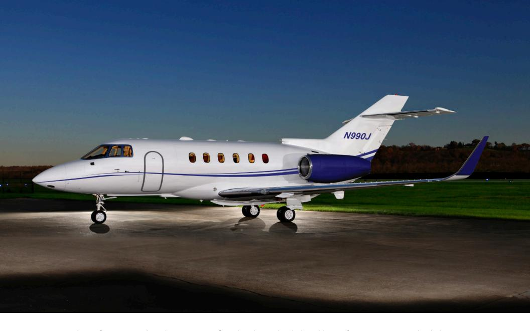
The performance and aesthetics are significantly enhanced with the addition of Aviation Partners Blended Winglets. N990J is up to 7 percent more fuel efficient, boasting an additional range of 180 NM at speeds 18 knots faster than the average 800XP.
