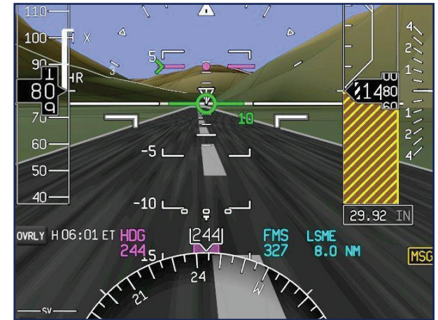
Approach with extended center-line, provided by the SmartView™ Synthetic Vision System, increases position awareness with respect to the landing environment.
