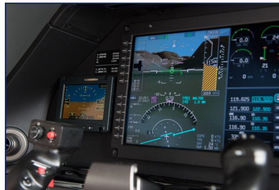
The SmartView™ Synthetic Vision System improves terrain/obstacle awareness by enabling early recognition of conflicting terrain and obstacle, particularly during instrument approaches.
