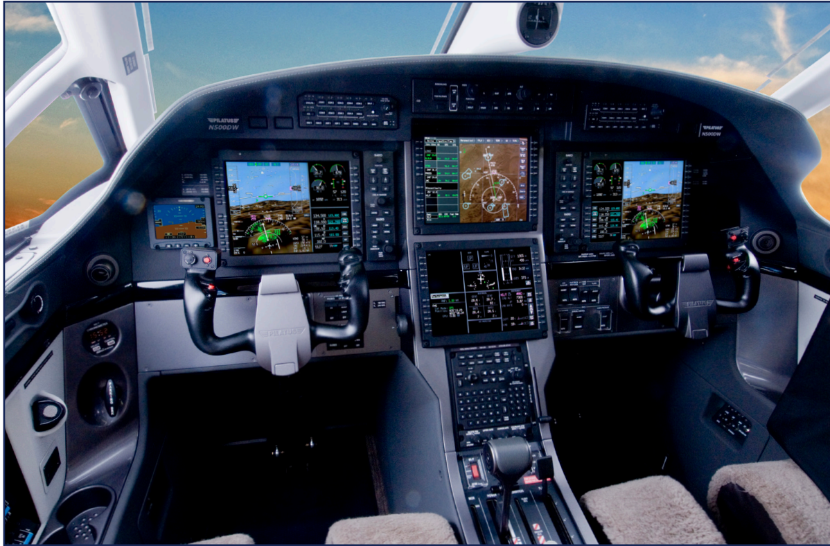
Approach with extended center-line, provided by the SmartView™ Synthetic Vision System, increases position awareness with respect to the landing environment.
