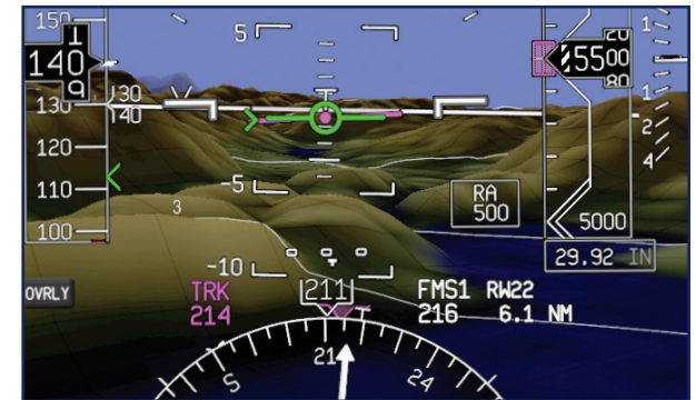
The SmartView™ Synthetic Vision System improves terrain/obstacle awareness by enabling early recognition of conflicting terrain and obstacle, particularly during instrument approaches.
