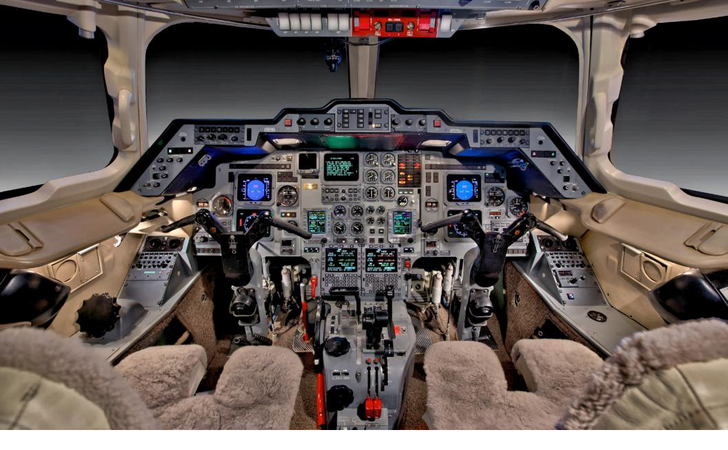
The 2020 compliant Primus II avionics platform features Dual Honeywell FMZ-2000 FMS Units with 6.0 software and ADS-B Out Version 2.
