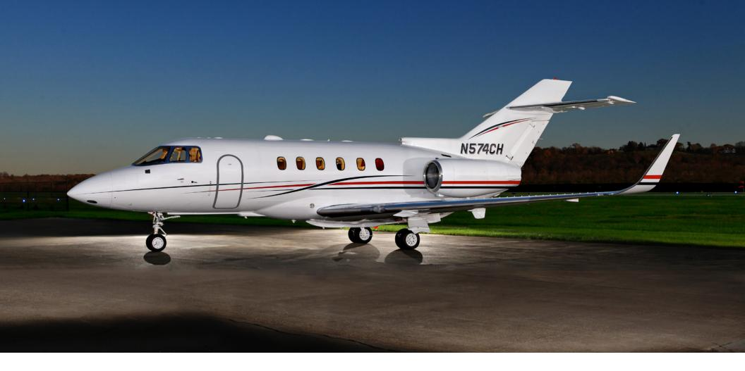
The performance and aesthetics are significantly enhanced with the addition of Aviation Partners Blended Winglets. As a result, SN 258540 is 7 percent more fuel efficient, boasting an additional range of 180 NM at speeds 18 knots faster than the average 800XP.
