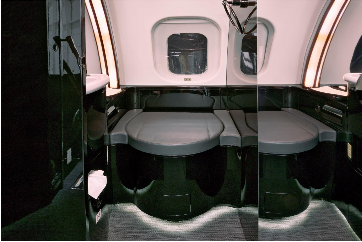
Forward Crew Lavatory (Vacuum Flush)
