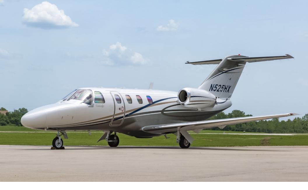
The CitationJet's unique wing maintains smooth, uninterrupted flow of air across a much greater portion of its surface than a conventional wing. This greatly reduces drag, and significantly enhances both performance and efficiency.
