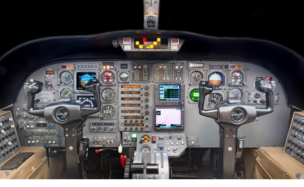
Certified for single-pilot operations, the Honeywell SPZ-5000 Avionics Suite is complemented by a BF Goodrich 497 Skywatch TCAS, Garmin GPS500W w/ WAAS, and GMX-200 Multi-Function Display.
