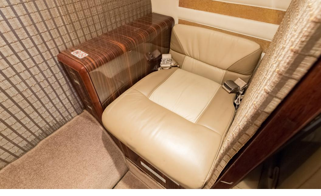
The aft lavatory seat is belted and certified for take-off and landing for a sixth passenger.
